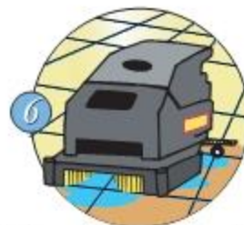
6 Scrub area with an automatic equipped with red pads, using medium pad pressure, with feed valve 3/4 open, squeegee down, and vacuum motor on.
