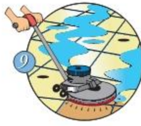
9 Scrub with circular scrubber, equipped with a red pad.
